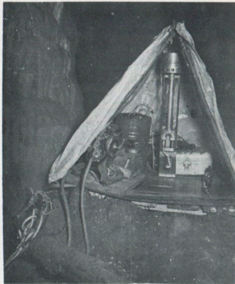
Figure 4. Tent for instruments in the cave. Telephone, box protecting the battery, thermistor psychrometer and remote control switch in aluminum box (1959).
